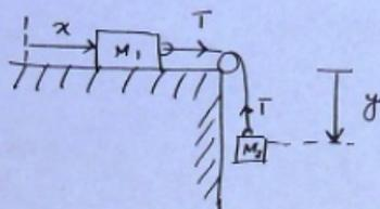
$$\ddot{x} = \ddot{y} \quad \text{---(i)} \quad T - M_2g = -M_2\ddot{y} \quad \text{---(ii)}$$
